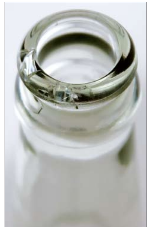
The HEUFT InLine checks the container finish three times straight away. The result: the detection accuracy is increased and false rejections are prevented even more effectively.
