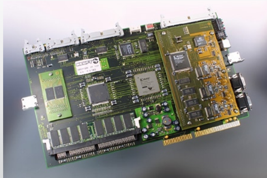
The HEUFT reflex image processing card
