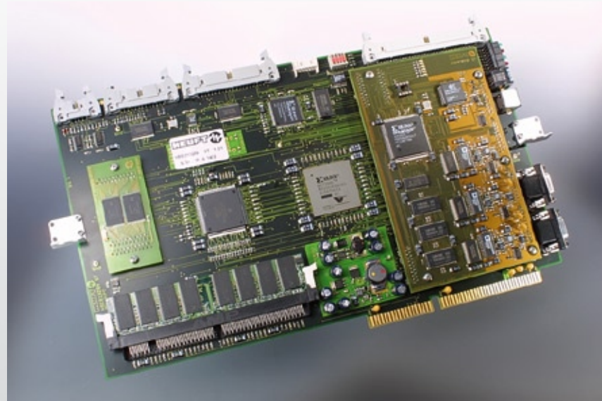
The HEUFT reflex image processing card
